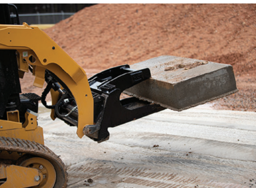
Concrete Slab Bucket
