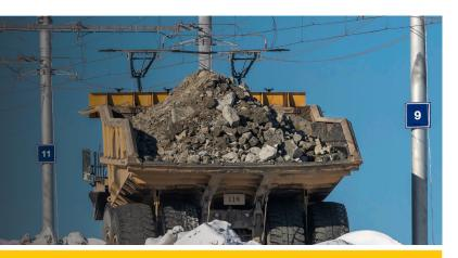
The Cat Trolley Assist System requires incremental truck iron and significant site infrastructure footprint to enable its operation. There are five key elements of the site infrastructure, they are: AC substation, DC substation(s), support poles, catenary lines, and the load height check. Site infrastructure for the trolley system must be provided by a third-party.
